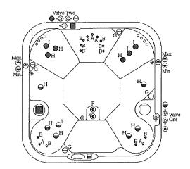
0 Hi-Flo Vortex Filter Auxiliary Filter Operator Panel Auxiliary Jet Control let Zone Selector Valve let Zone Air Control © (<del>A</del>) Ozone let Neck Jet Selector Valve Cascade Neck Jet A B Micro Boost Jet
